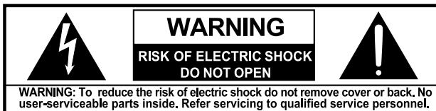
The lightning flash with arrow-head within a triangle is intended to tell the user that parts inside the product are a risk of electric shock to persons.
